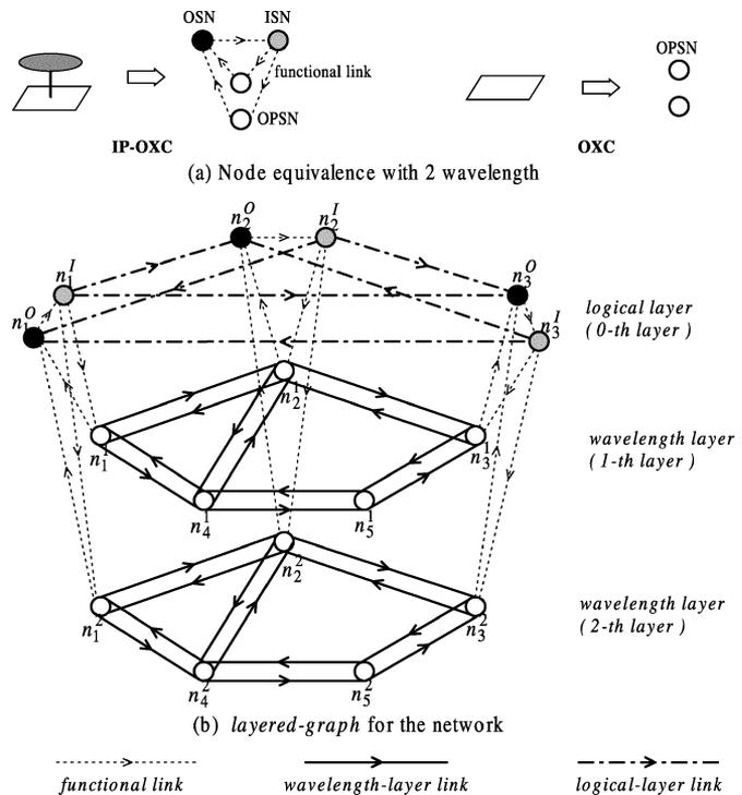
Fig. 2. Layered-graph for the sample network shown in Fig. 1. (a) Equivalence relations of IP-OXC and OXC. (b) Layered-graph for the network. In the layered-graph, the zeroth layer represents the logical layer and the  $w$ th layer indicates the  $w$ th wavelength layer ( $1 \leq w \leq 2$ ).
