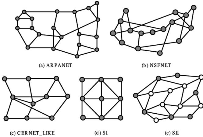
Fig. 3. Sample networks used in the simulations. (a) 20-node ARPANET. (b) 16-node NSFNET. (c) 10-node CERNET\_Like. (d) 9-node Sample I. (e) 15-node Sample II. Each node with an open circle in the networks denotes an OXC, and each node with a gray circle denotes an IP-OXC.
